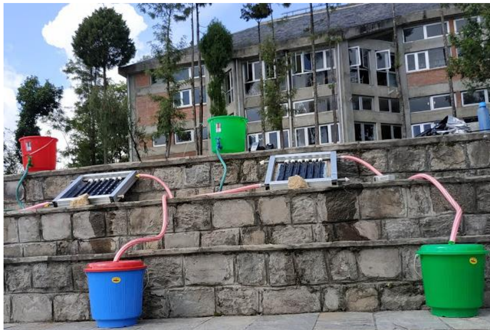
Figure 1. Performance evaluation of solar water heating system fabricated using black paint (left) and black nickel selective coating.
